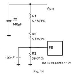
The LD7268A could sense output voltage by using an output resistor divider or a high voltage zener diode.
