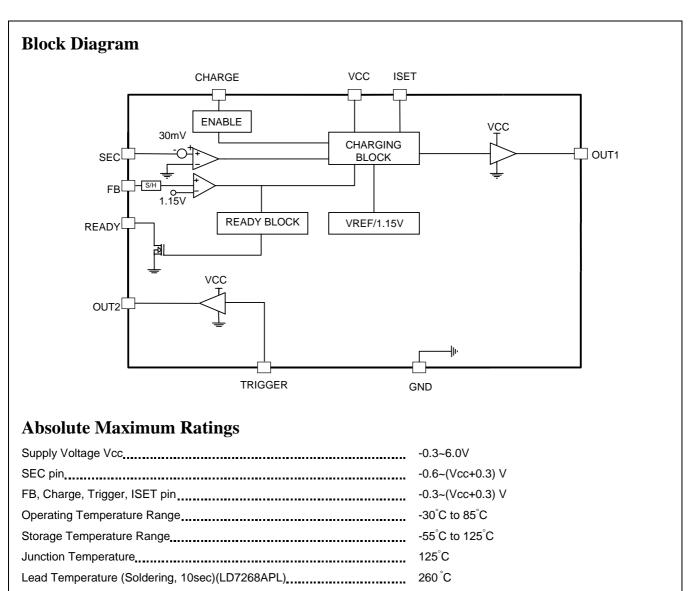
stresses beyond the ratings specified in "Absolute Maximum Ratings" may cause permanent damage to the device. This is a stress only rating and operation of the device at these or any other conditions above those indicated in the operational sections of this specification is not implied.
