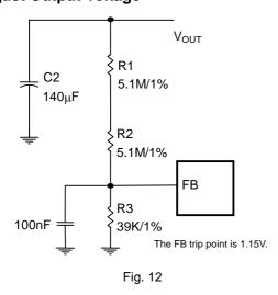
The LD7261A could sense output voltage by using an output resistor divider. The Fig. 12 shows the application circuit of resistor divider.
