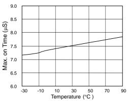
Fig. 9 Max on Time vs. Temperature
