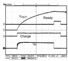
Fig. 3 Charging Waveform V<sub>IN</sub>=1.8V
