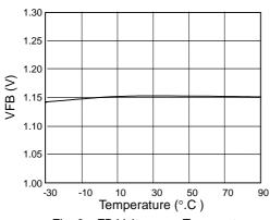
Fig. 8 FB Voltage vs. Temperature
