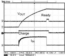
Fig. 2 Charging Waveform V<sub>IN</sub>=3V
