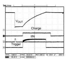
Fig. 4 Charging Waveform  $V_{IN}$ =3V
