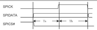
Figure 4 SPI Interface Timing Diagram
