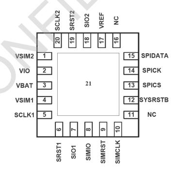
Figure 2 ft6188 QFN-20 Top View
