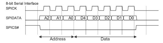
Figure 3 SPI Interface Date Transmission Timings
