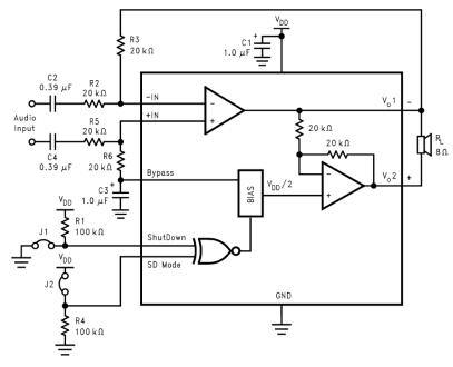
Figure 4. DIFFERENTIAL AMPLIFIER CONFIGURATION FOR ft690
