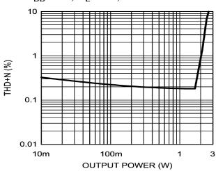
THD+N+N vs Output Power  $V_{DD}$  = 3V,  $R_L$  =  $4\Omega$ , and f = 1kHz
