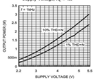
Output Power vs Supply Voltage,  $R_L = 8\Omega$
