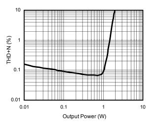
THD+N+N vs Output Power Vdd=3V, RL=8  $\Omega$  , f=1 KHz
