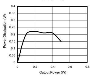
Power Dissipation vs Output Power Vdd=2.6V, RL=8  $\Omega$
