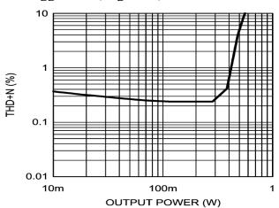
THD+N+N vs Output Power Vdd=2.6V, RL=8  $\Omega$  , f=1KHz
