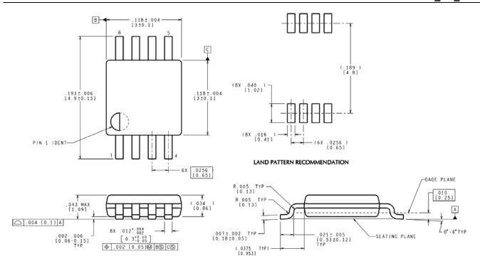
Figure 6. MSOP Package Physical Dimension
