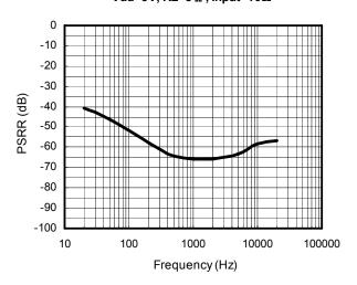
PSRR vs Frequency Vdd=3V, RL=8  $\Omega$  , Input=10 $\Omega$
