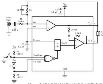
Figure 3. HIGHER GAIN AUDIO AMPLIFIER
