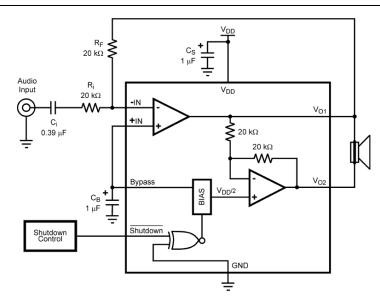
Figure 2.Typical Audio Amplifier Application Circuit (MSOP and WCSP)
