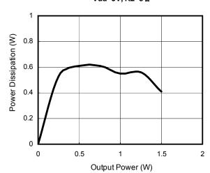
Power Dissipation vs Output Power Vdd=3V, RL=8  $\Omega$
