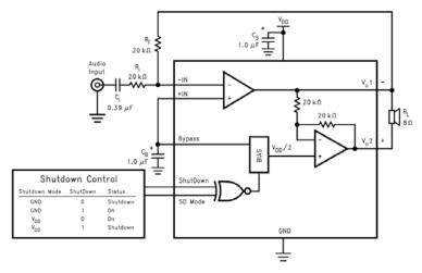
Figure 1. Typical Audio Amplifier Application Circuit (DFN)
