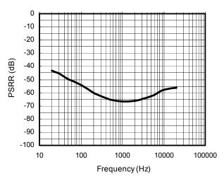
PSRR vs Frequency Vdd=2.6V, RL=8  $\Omega$  , Input=10 $\Omega$
