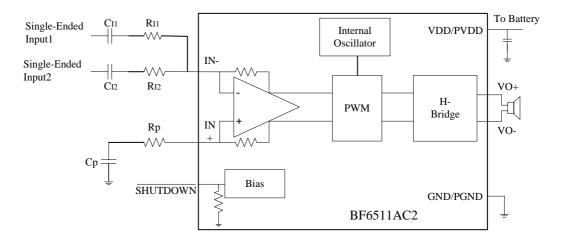
Figure 6. Application Schematic with BF6511AC2 Summing Two Single-Ended Inputs
