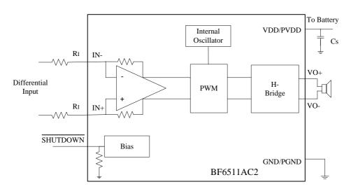
Figure 1. Typical BF6511AC2 Application Schematic with Differential Input for a Wireless Phone
