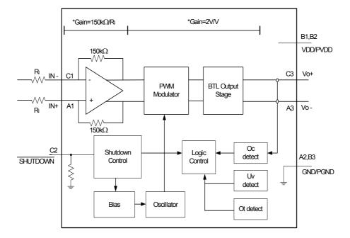
Notes: Total gain =2\*150 kΩ/R<sub>1</sub> Oc: Over Current Uv: Under Voltage Ot: Over Temperature
