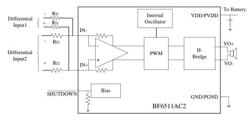
Figure 4. Application Schematic with BF6511AC2 Summing Two Differential Inputs
