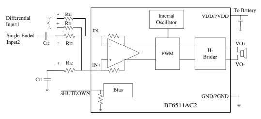
Figure 5. Application Schematic with BF6511AC2 Summing Differential Input and Single-Ended Input Signals
