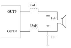
Figure 8. Typical LC Output Filter, Cutoff Frequency of 27 kHz
