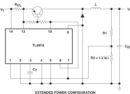
(using external transistor)
