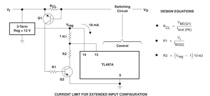
Figure 4. Extended Input Voltage Range (V<sub>I</sub> > 12 V)
