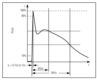
Figure 5b. IEC 1000-4-2 ESD Generator Current Waveform
