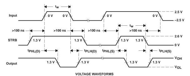
NOTES: A. The pulse generators have the following characteristics:  $Z_O = 50~\Omega$ ,  $t_f \le 10$  ns,  $t_W = 0.5~\pm 0.1~\mu$ s, PRR  $\le 1~MHz$ .
