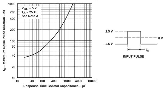
NOTE A: Figure 11 shows the maximum duration of the illustrated pulse that can be applied differently without the output changing from the low to high level.
