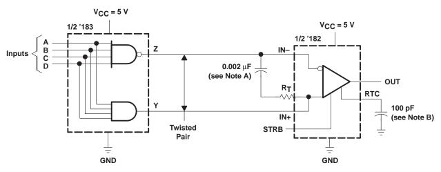
NOTES: A. When the inputs are open circuited, the output is high. A capacitor may be used for dc isolation of the line-terminating resistor. At the frequency of operation, the impedance of the capacitor should be relatively small.
