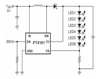
Figure 1. Li-Ion Driver for Six White LEDs
