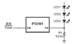
Figure 9. Dimming Control Using a PWM Signal
