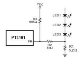
Figure 8. Dimming Control Using a DC Voltage
