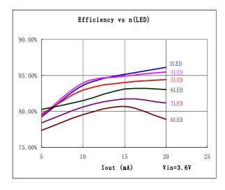
Figure 2. Efficiency vs Number of LEDs
