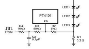
Figure 10. Dimming Control Using a Filtered PWM Signal
