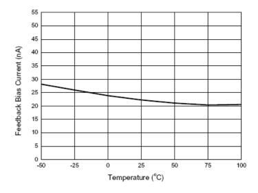
Figure 7. Feedback Bias Current vs. Temperature
