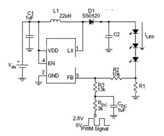
Figure 6. Filtered PWM Signal for LED Dimming Control
