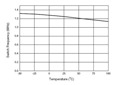
Figure 6. Switch Frequency vs. Temperature
