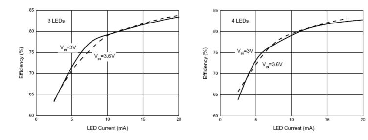
Figure 10. Efficiency vs. LED Current
