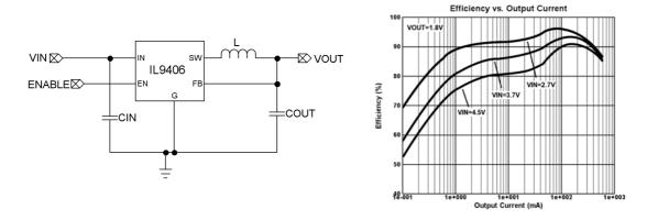
Figure 1. Typical Application Circuit and Efficiency
