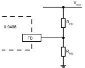
Figure 3. Output Voltage Programming
