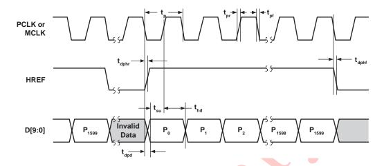
Figure 9 SVGA Line/Pixel Output Timing
