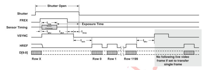
Figure 13 Frame Exposure Mode Timing with EXPSTB Asserted
