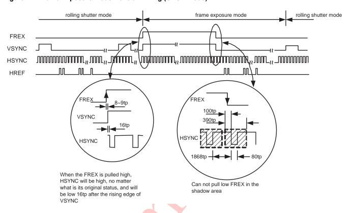
Figure 15 Frame Exposure Mode Control Timing (SVGA Mode)
