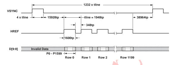
Figure 11 SVGA Frame Timing
