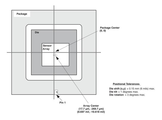
**Important:** Most optical systems invert and mirror the image so the chip is usually mounted on the board with pin 1 (SVDD) down as shown.
