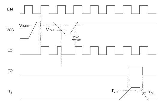
After UVLO is released, IC operation is started by the first rising edge of input
