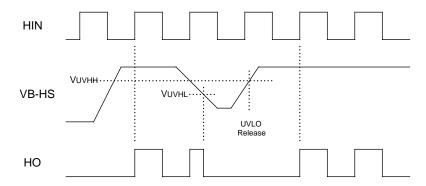
After UVLO is released, IC operation is started by the first rising edge of input
