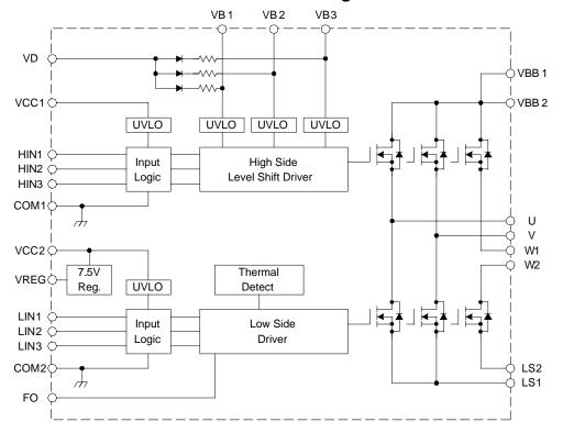
Figure 1. Driver block diagram.
